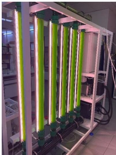
Figure 1. Pilot-scale tubular airlift photobioreactor installed in CETH facilities.
